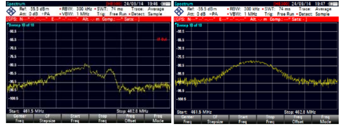
Fig. 6 Left: interfered radio signal; right: non-interfered signal.
