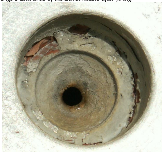
Fig. 8 Exit area of the Laval nozzle after firing
