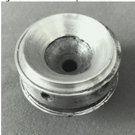
Fig. 6 Steel nozzle and composite insert.
