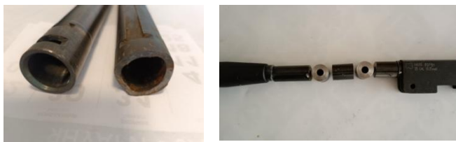
Fig. 1 Weapon components showing defects of different types a) original and broken b) air rifle barrel, distorted pistons
