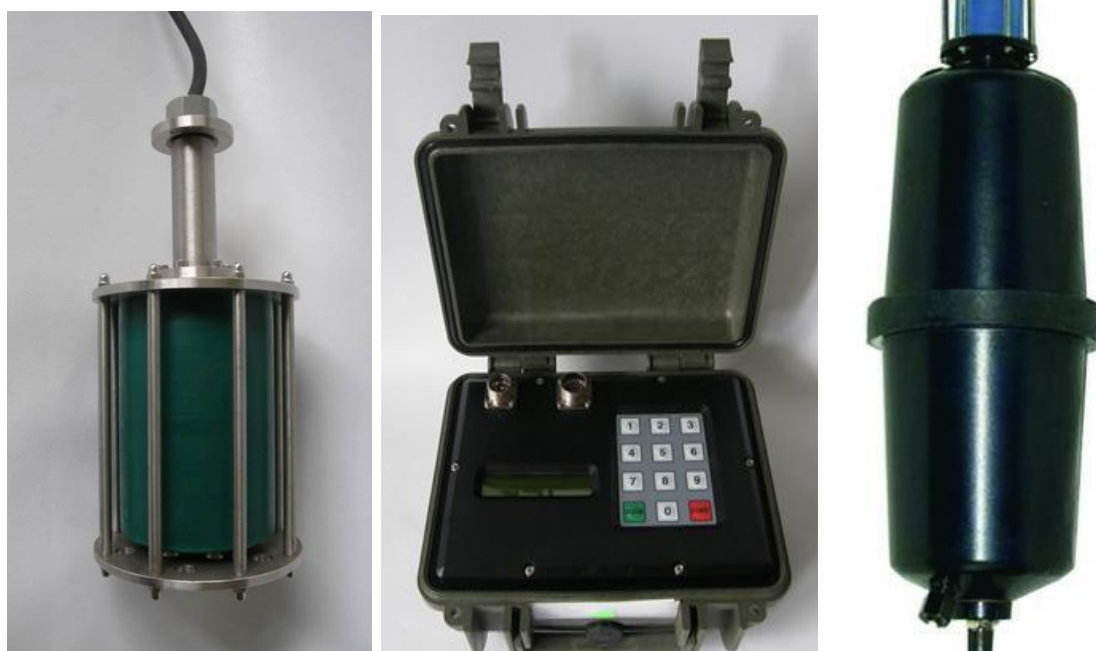
Fig. 1. Management and control system of explosive devices : on the left - emitting antenna, in the center - command electronic unit and on the right - receiving device
