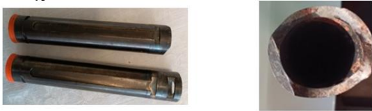
Fig. 2 General view of an air rifle "piston" type part - new part and one with a tear defect. The location of the fracture coincides with a structural opening
